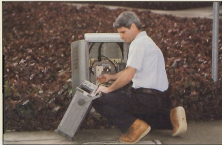
Using a credit-card-size ROM card, a technician can customize HP's 8591A portable spectrum analyzer to measure the quality of cable TV signals.
